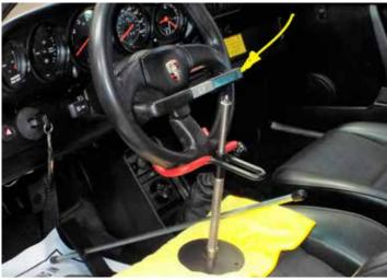
was a steering wheel lock and a level he uses to keep the steering wheel straight that he said many do not use and instead do it by eye. I like the level idea too.
