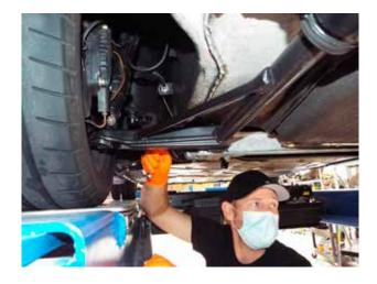
I thought having a shock tower brace would complicate the alignment but in actuality Adam was able to utilize it to help make adjustments. Adam proceeded to get in the driver seat several times through the process making adjustments and rechecking. The goal on the front was 1.6 mm toe with him in the car. And this is where again the
